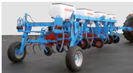
8-row rigid TIP 5" cultivator with 70cm inter-row spacing during transport
