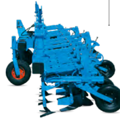
12-row front-mounted cultivator with "inverted units" with 45cm inter-row spacing
