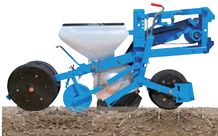
MECA V4 METERING UNIT 260x100 front wheel - Front gauge wheel
