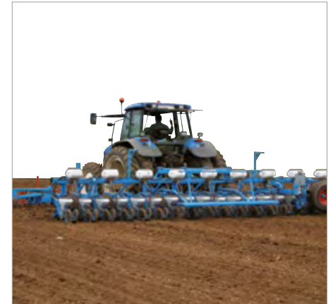
MECA V4 18-row triple-bar rigid planter with Microsem and transport carriage
