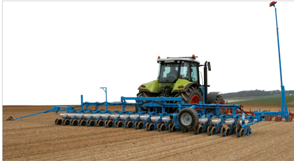
MECA V4 18-row triple-bar rigid planter with transport carriage
