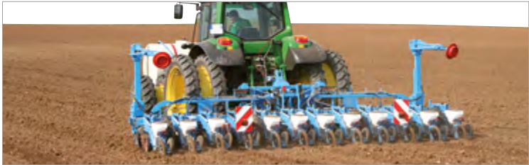
MECA V4 12-row double-bar folding planter
